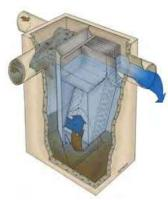
Vortex Hydrodynamic Separator Source: Stormwater Solutions
