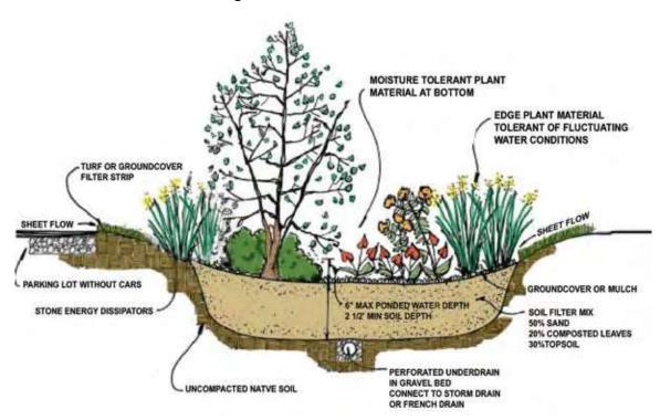
Figure 7.6 Schematic of a technically engineered bioretention area MAX. PONDED WATER DEPTH (6"-18") MAX 3:1 SIDE SLOPES (TYP.) LEAF COMPOST OR SHREDDED HARDWOOD. AVOID WOOD CHIPS. POSITIVE OVERFLOW PLANTING 18-48\* SYSTEM SOIL WRAP BED WITH NON-WOVEN GEOTEXTILE STORAGE BED 6-12" 6 LF OF 10"Ø PERF. PIPE (OPTIONAL) 12" MIN. SUMP OPTIONAL UNIFORMLY GRADED CLEAN AGGREGATE OR CLEAN WASHED SAND
