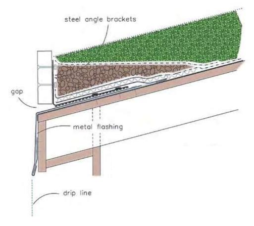
Example eave detail for sloped roof
