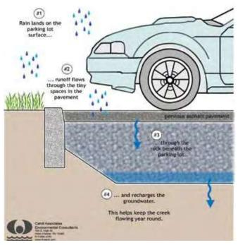
Pervious pavement with infiltration schematic
