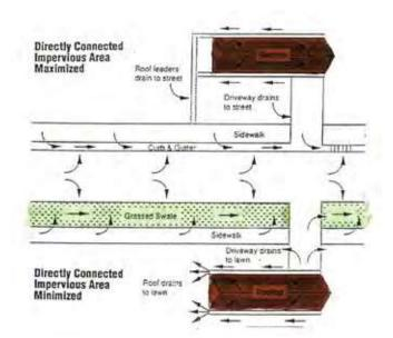
Difference between maximizing and minimizing runoff Source – Center for Watershed Protection
