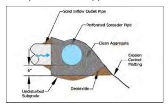
Level spreader with geotextile surrounding the aggregate helping to create a sloped area.
