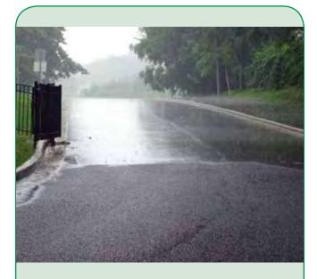
The City of Battle Creek Willard Beach Park Project showcases LID practices to the community by installing rain gardens and porous asphalt throughout the park roadway system. During a rainstorm, notice the amount of runoff from the traditional asphalt (top) versus the porous asphalt at the start of the park (bottom). These BMPs address both stormwater quantity and temperature concerns that are often associated with roadway runoff. Source: City of Battle Creek
