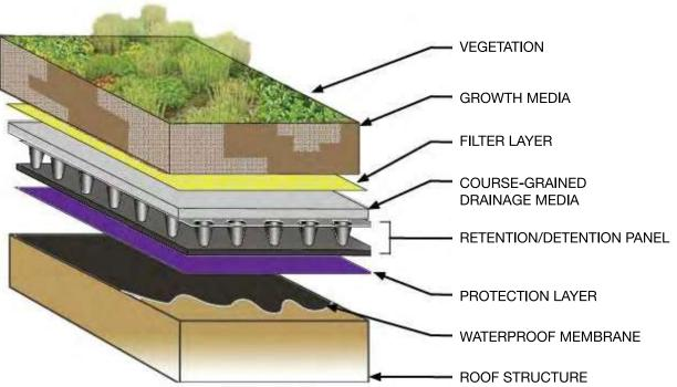
storm events relatively slowly. If overflow is directed to an infiltration system, the discharge can be infiltrated efficiently as the system has more time to absorb water as it is slowly released from the roof. Vegetated roof covers improve the efficiency of infiltration devices by:
