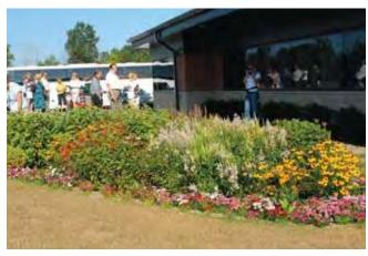
Bioretention is one variation of an infiltration BMP, such as this rain garden at the Macomb County Public Works Building
