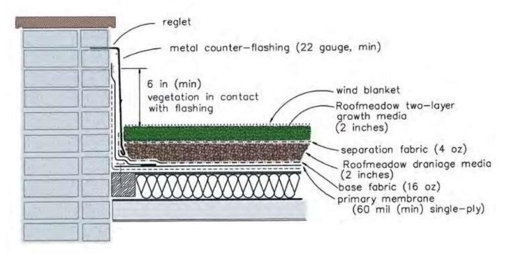
Example parapet flashing detail for a flat roof
