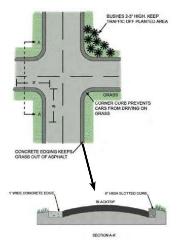
Curb cuts as a method of stormwater disconnection Source: Center for Watershed Protection, modified by Cahill Associates, 2008
