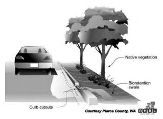
Curb cut-outs allow stormwater runoff from a parking lot to flow into a bioretention swale
