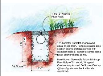
Level spreader schematic
