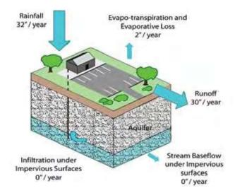
• Degradation of the stream channel. One result of runoff can be more water moving at higher velocities through stream channels. This condition is called "flashy flows" and happens at increased frequency as an area is developed. As a result, both the streambank and stream bed are eroded more frequently. This can result in widening and deepening the channel, as well as a decline in stream substrate quality, and degradation of habitat.
