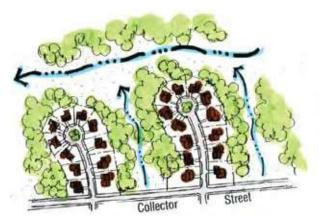
Natural drainage features can guide the design Source: Delaware Department of Natural Resources and Environmental Control - Conservation Design for Stormwater Management
