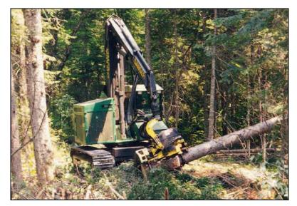
Figure 3. An Example of a Knuckleboom Harvester.
