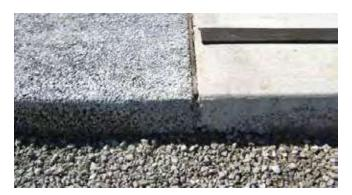
Pervious and impervious concrete
