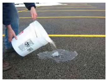
Water on Porous Asphalt
